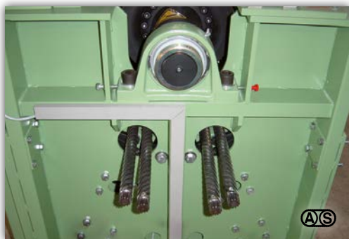
Lateral removal of the flex bars (the flex bars can also be removed from above)
