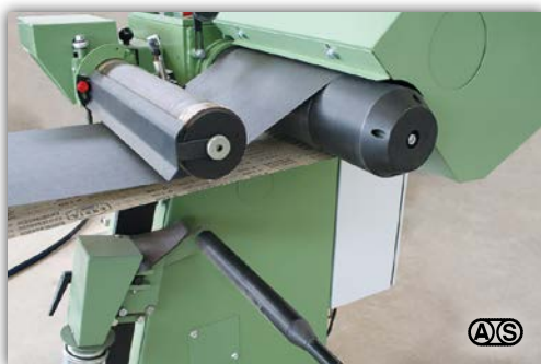
Cutting cylinder with automatic belt guiding system and short belt stretcher
